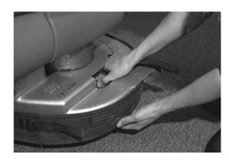
6. Pull the brush/pad driver out from under the scrub head.
