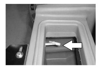
A vacuum fan filter is located in the recovery tank. Remove and clean this filter daily. Clean by shaking dust or rinsing pleats with low pressure water.
