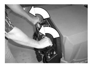
Turning: Push the machine in the direction of the turn with the steering handles. The machine will turn on the swivel casters.
