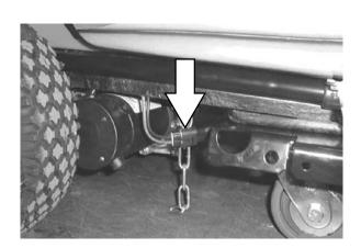
4. Lower the scrub head with the brushes or pad drivers installed, lower the squeegee when transporting the machine. Block the machine tires and tie down the machine to the truck or trailer before transporting.
