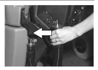
12. Pull up on the support arm and lower the solution tank. Push the stop arm in to completely lower the solution tank.
