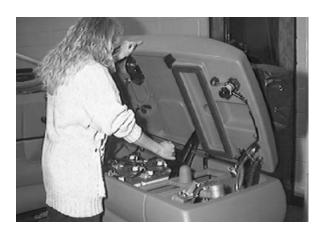
13. Cylindrical scrub head: Remove and clean the debris trough. Place the trough back in the scrub head.
