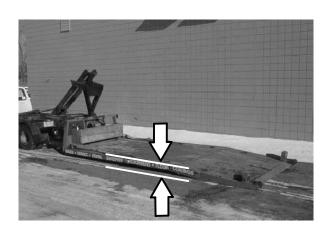
To winch the machine onto the truck or trailer, attach the winching chains to the rear tie down locations on either side of the machine frame by the rear casters.
