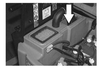
Rinse off the float sensor on the side of the recovery tank.
