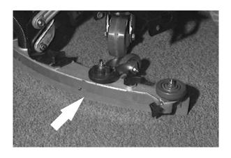
If the deflection is not the same over the full length of the blade, turn the squeegee leveling bolt counter-clockwise to increase the deflection at the ends of the squeegee.
