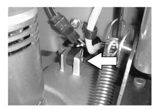
8. Mark the location of the actuator tube on the actuator shaft before disconnecting the actuator. Disconnect the actuator from the scrub head by removing the clevis pin.
