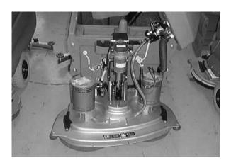
4. Disconnect the solution line from the scrub head tee fitting.
