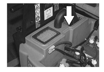
Rinse and wipe off the sensors daily on machines with float sensors installed inside the recovery tank.
