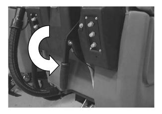
7. CONVENTIONAL SCRUBBING: Adjust the solution flow to the floor as needed.
