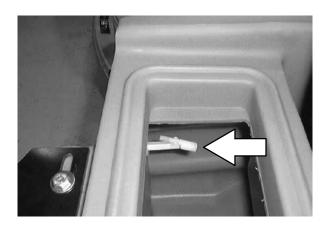
10. Remove and clean the vacuum fan filter located in the recovery tank. Clean by shaking dust or rinsing pleats with low pressure water. Insert the filter back in to the recovery tank when finished.
