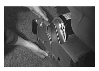
B. While holding the flat end of the idler shaft with a wrench, loosen the mounting screw on the outside of the idler door.
