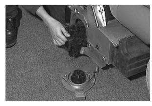
Insert the Idler plug of the idler door into the brush.
