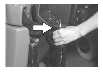
5. Remove the recovery tank drain hose plug while holding the hose up, then slowly lower the drain hose to the floor drain or sink.
