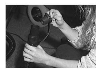
6. Check the solution tank, and empty any remaining solution with the solution tank drain hose.
