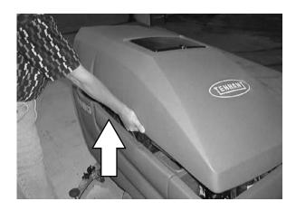
Place the FaST PAK carton in the carton holder under the front cover of the machine. Connect the supply hose to the FaST PAK bag.
