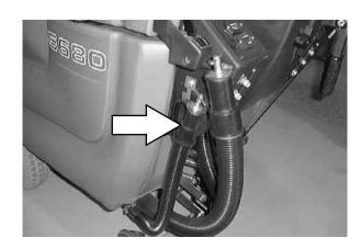
7. Lift the solution tank to reach the recovery tank.
