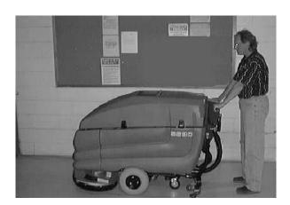
3. Heavy Scrub Mode only: With the scrub head in the up position, pull out on the scrub head strap, until the scrub head drops into place.
