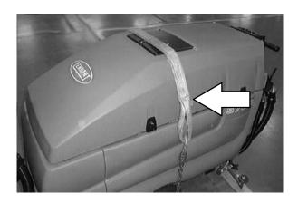
The rear tie-down locations are on either side of the machine frame by the rear casters.
