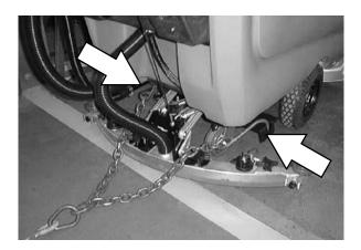
2. Unplug the drive motor from the electrical harness before attempting to winch the machine. The machine will become easier to maneuver when it is unplugged.
