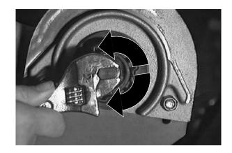
The brush patterns should be the same width. If one is narrower then the other, loosen the jam nut on the adjustment screw located on the top of the scrub head.
