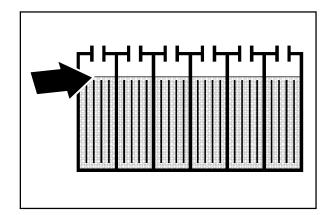
Measuring the specific gravity, using a hydrometer, is a way to determine the charge level and condition of the batteries. If one or more of the battery cells test lower than the other battery cells (0.050 or more), the cell is damaged, shorted, or is about to fail.
