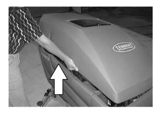
4. Check the water level in all the battery cells. If the level is low, add just enough distilled water to cover the plates. DO NOT OVERFILL. The batteries can overflow during charging due to expansion.
