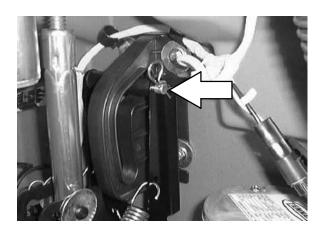
7. Disconnect the lift arms from the scrub head by removing the two clevis pins.
