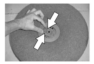
9. Flip or replace the scrub pad, center the scrub pad on the pad driver.
