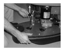
Brush Deck may be tilted up for easier brush installation/removal & to clear steep ramps. Lift the handle on the upper lever which connects the brush deck to the machine, tilt the deck up, release the handle & the lever will lock into place. Lift the handle again to move the deck back to horizontal.
