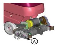
1. Raise brush deck. Unscrew the knob on the right side of the deck as shown above. Pull open the Hinged Cover (A).
