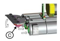
3. Insert Idle Hubs (C) into the brushes while closing the hinged cover. Tighten the knob on the cover by hand, ensuring that the hinged idle cover is flush to the deck.
