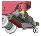
2. The drive side of each brush has a black end-cap with teeth. Insert the drive side of the brush through the opening until engaged on to the Drive Hub (B).
