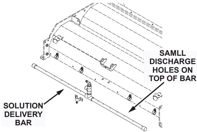
Fig. 1: Solution Delivery Bar shown with holes
