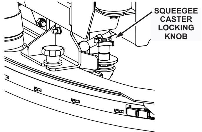
Fig. 1: Adjusting the Rear Squeegee Blade Flair
