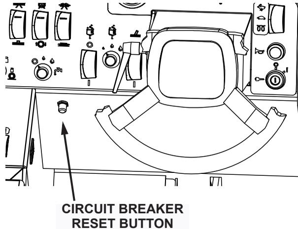
Fig. 1: Circuit Breaker location
