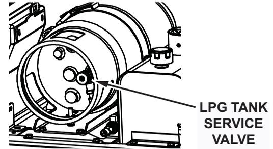
Fig. 1: LPG Tank - Location of Service Valve
