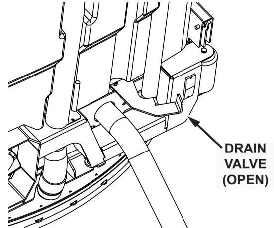
Fig. 2: Drain Valve
