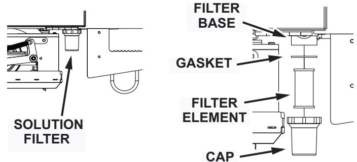
Fig. 2: Water Solution Filter with Exploded view
