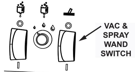
Fig. 2: Vacuum and Spray Wand Switch
