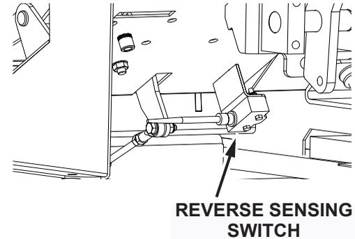
Fig. 3: Reverse Sensing Switch location
