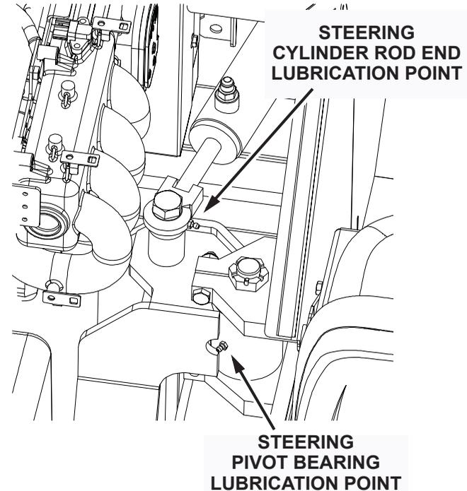
Fig. 1: Lubrication Points
