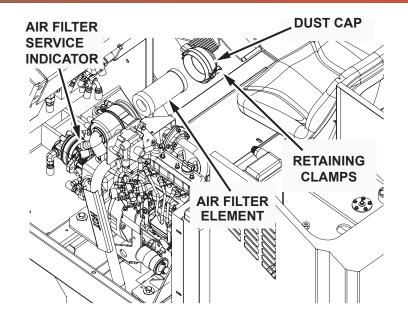
NOTE: The indicator may return to the nonviable position when the engine is shut off. To check, reset indicator and turn on the engine, if it locks in visible position again clean or change element.
