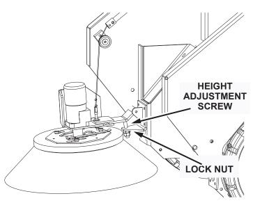
4. Side Broom should make contact with floor in the "10 to 3 o'clock position.
