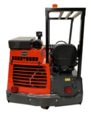
**Common Safety Options** Overhead guard, flashing light, and full enclosed cab as an option (MERV-17 HEPA shown) **81.00"** (height to top of overhead guard/cab)
